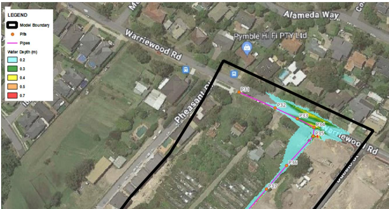
Figure 1: PMF inundation extent on Warriewood Road
