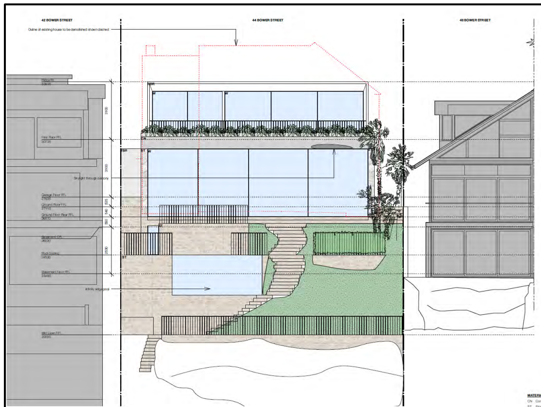
Figure 22: Extract of the rear elevation plan. The red dashed line indicates the bulk of the existing dwelling. The proposed dwelling will have a significantly reduced bulk compared to the existing dwelling.
