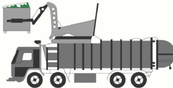
Front-lift-loading waste collection vehicle
