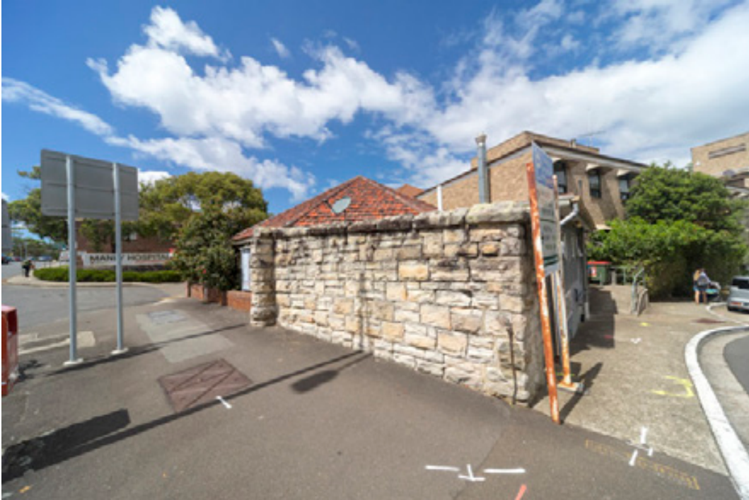
Figure 97: The Kiosk from the north-west. Note the andstone wall shown here is of recent construction (possibly using stone from the demolished section of the eastern boundary wall of the core hospital site). Building 3 is visible beyond at right.
