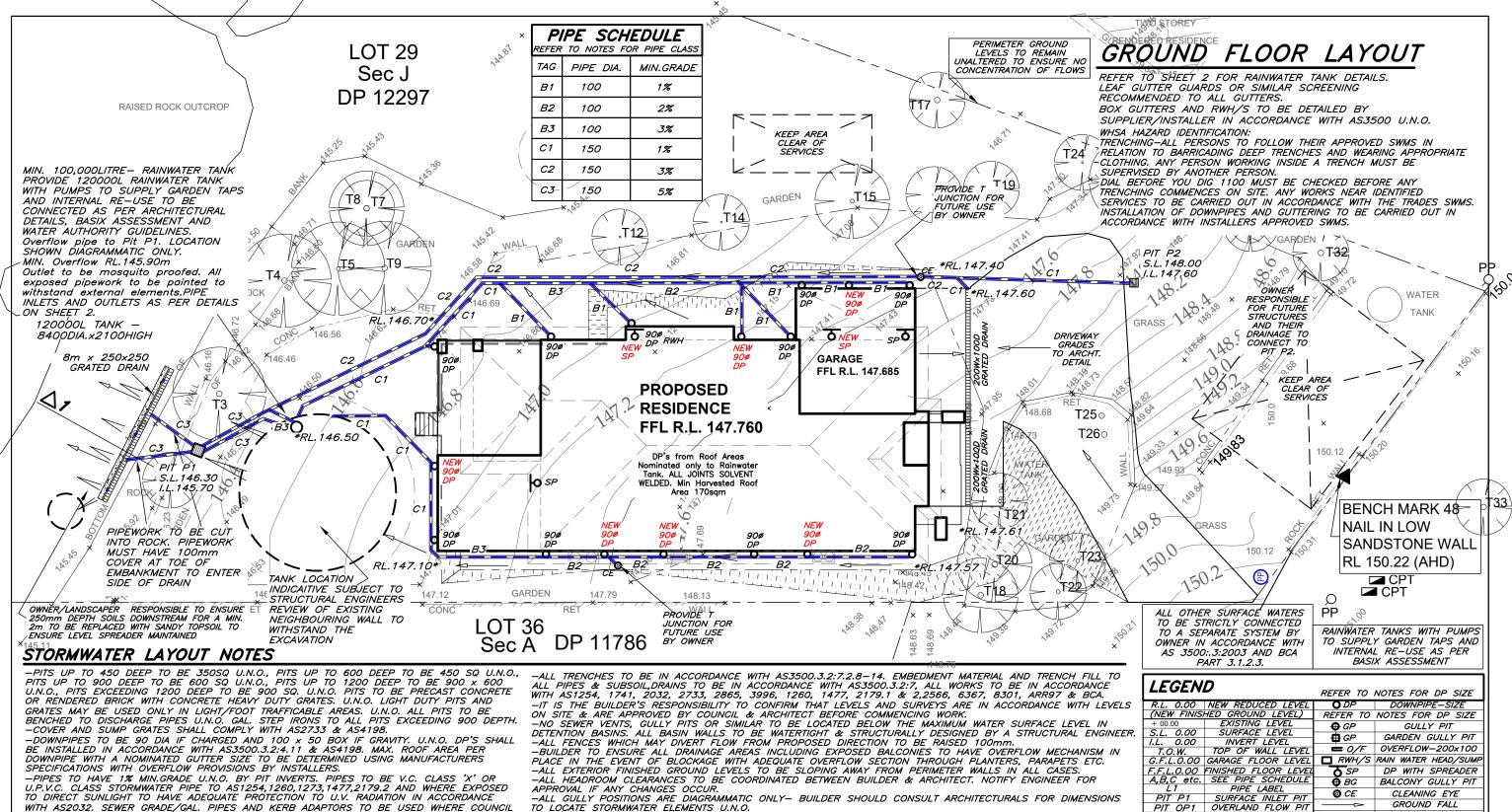
WITH AS2032. SEWER GRADE/GAL. PIPES AND KERB ADAPTORS TO BE USED WHERE COUNCIL
