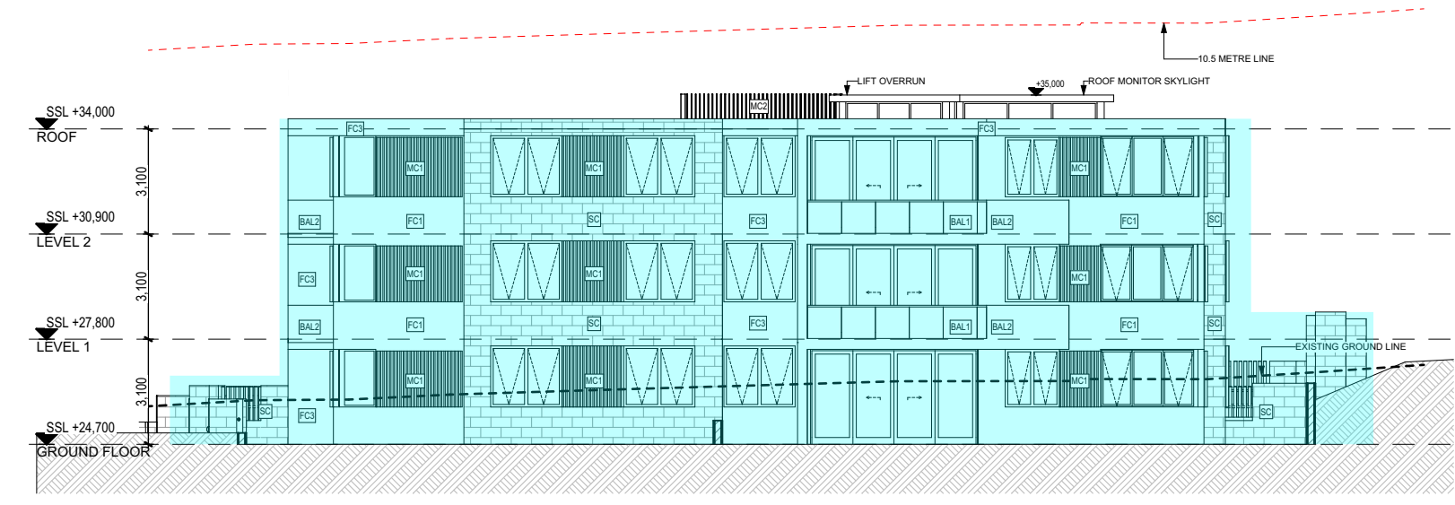
8 West Elevation - Building B Scale @ A1 = 1:200
