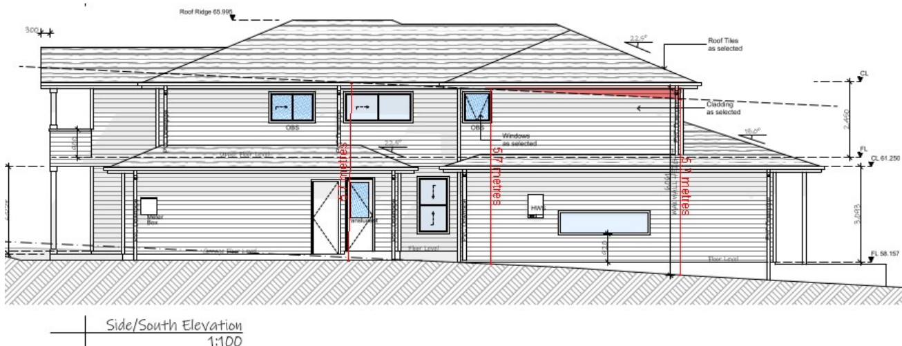
Figure 2: Side boundary envelope breach on the southern elevation shown in pink
