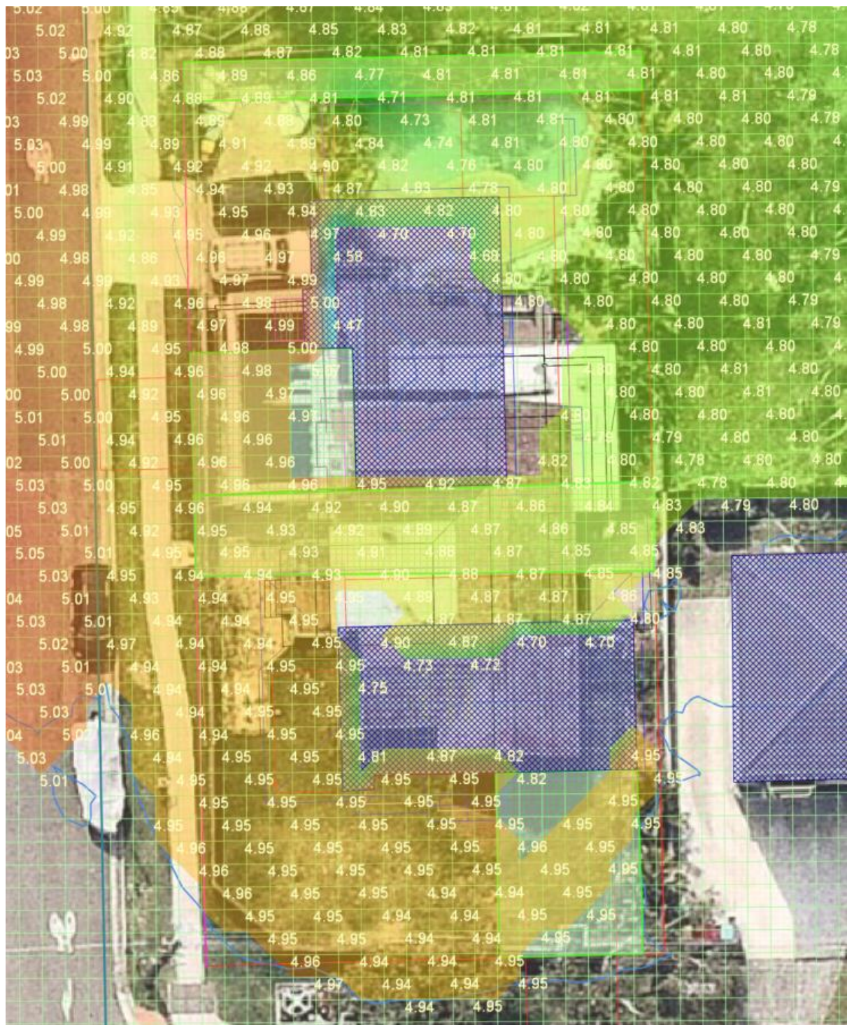
Figure 12: Post- development Water Elevation – 1% AEP
