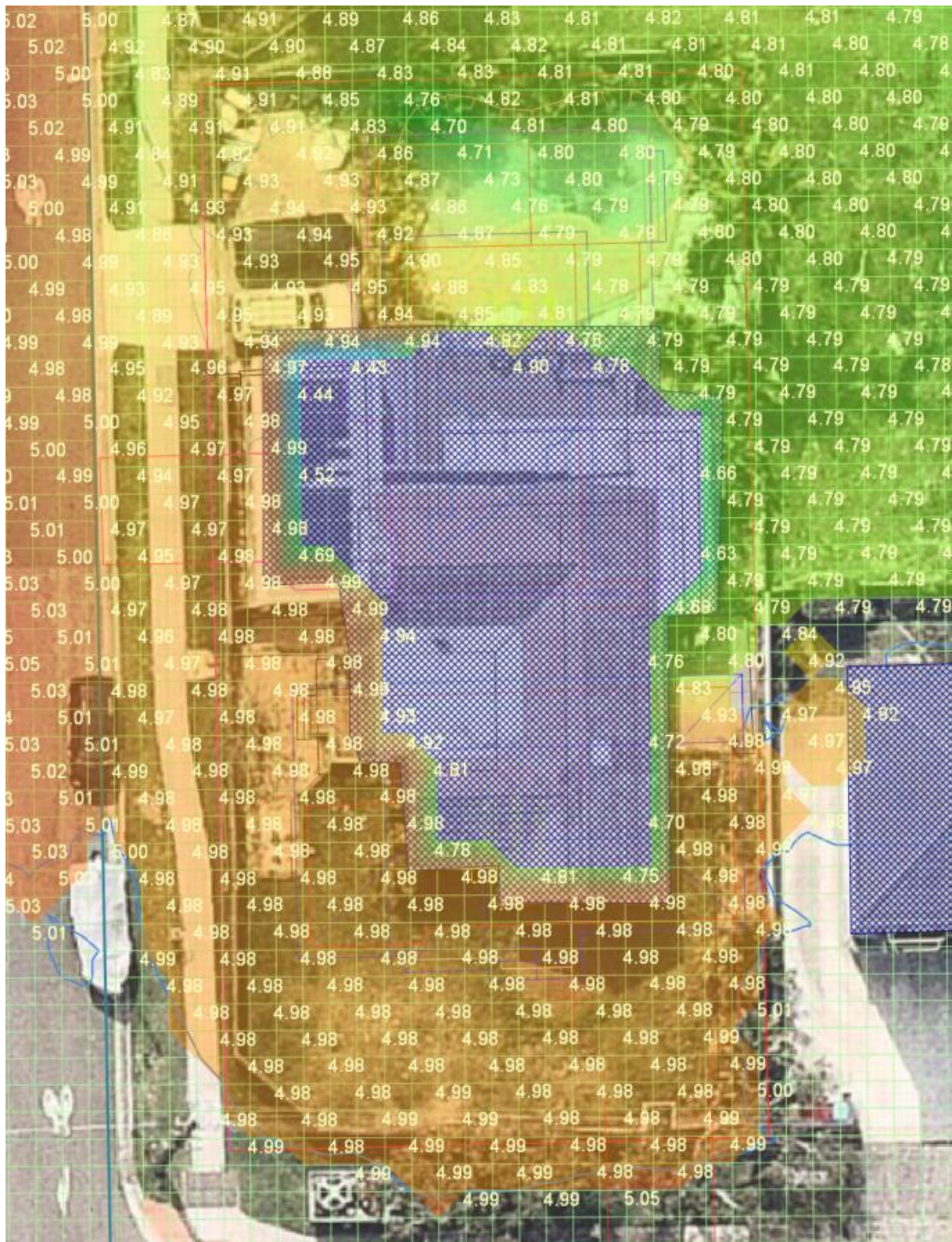
Figure 9: Pre-development Water Elevation – 1% AEP
