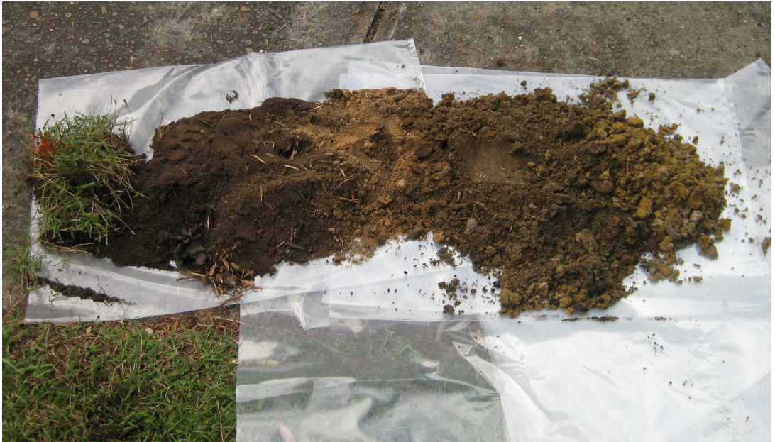
Photograph C1 – View of soils excavated from Borehole BH1, with the top of the soil profile commencing from the left of the field of view.
