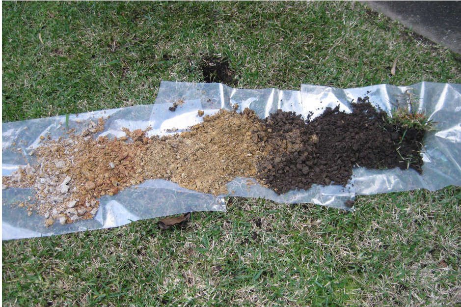
Photograph C2 – View of soils excavated from Borehole BH102, with the top of the soil profile commencing from the right of the field of view.
