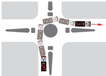
Example of a swept path as applied to a roundabout. The distance between inner and outer turning arcs allows for expected vehicle body swing of front and rear overhanging sections (the swept path).
