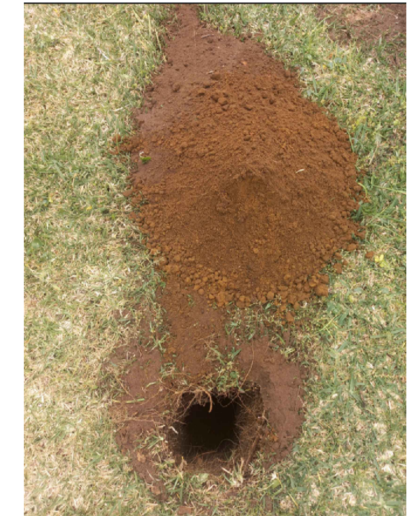
SUB STRATA ABSORPTION DETAIL COARSE SAND as per BCE pty ltd site investigation 25 / 09 / 2024
