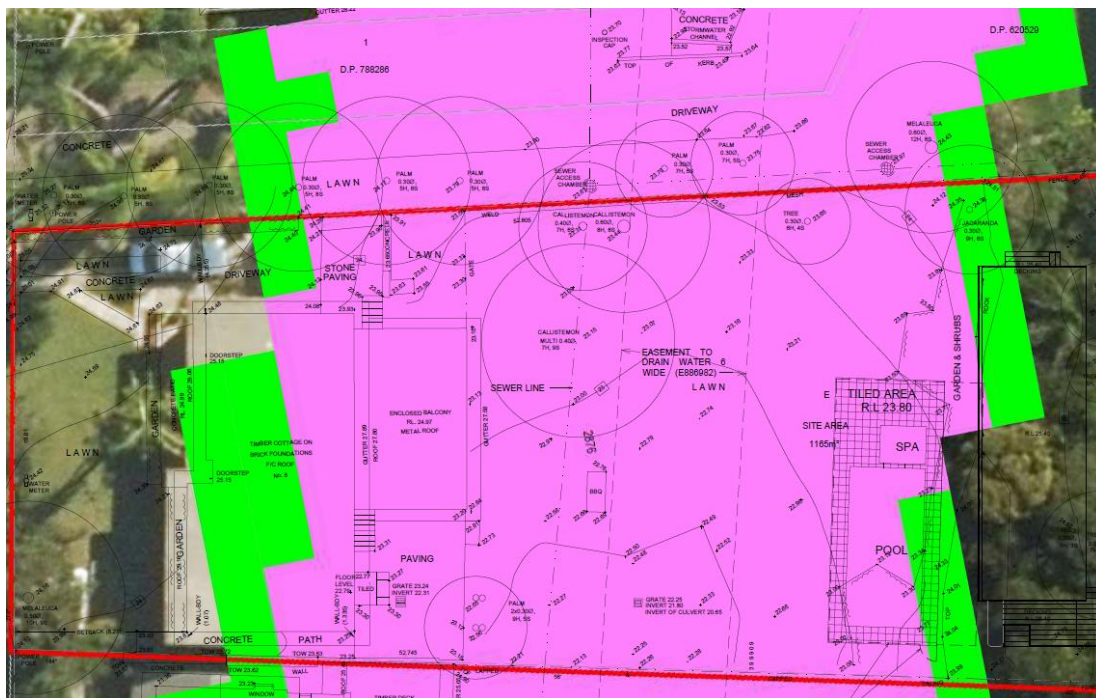
Figure 7: Ground floor plan overlay with PMF Flood Hydraulic Category map
