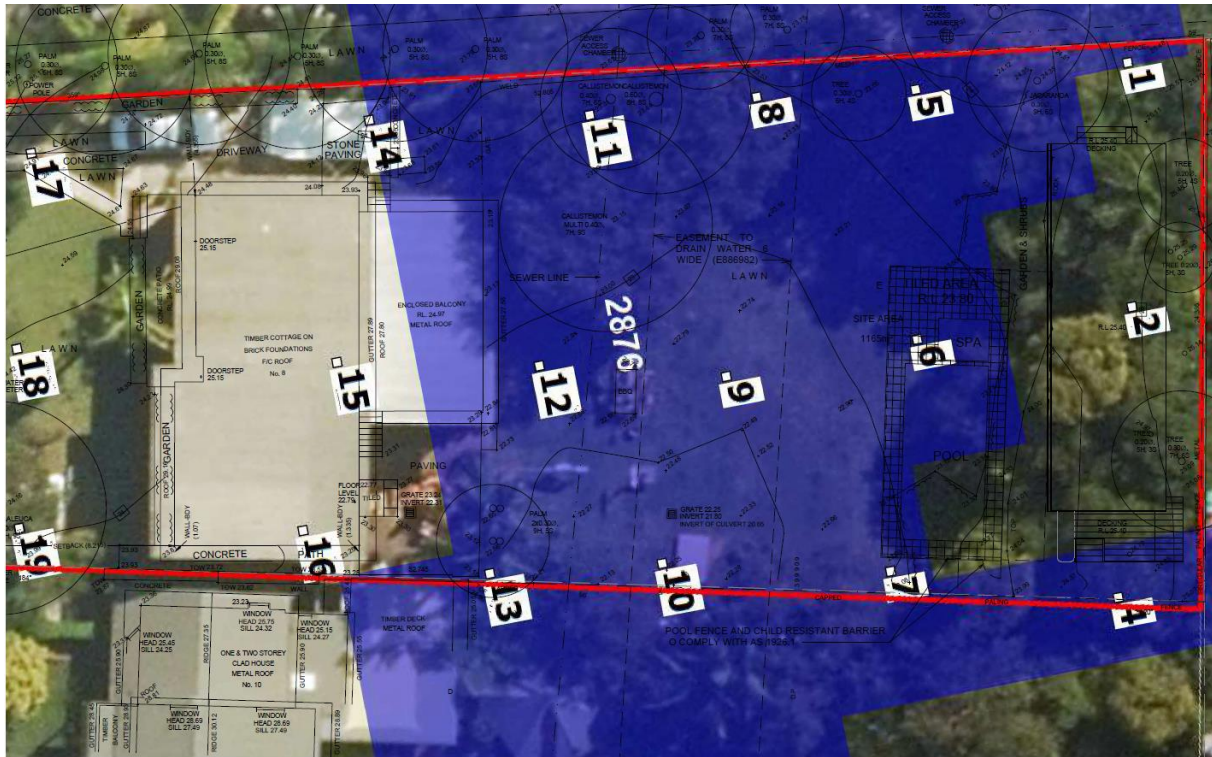
Figure 2: Ground floor plan overlay with 1% AEP Flood level points
