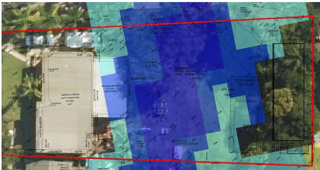
Figure 3: Ground floor plan overlay with 1% AEP Flood hazard map
