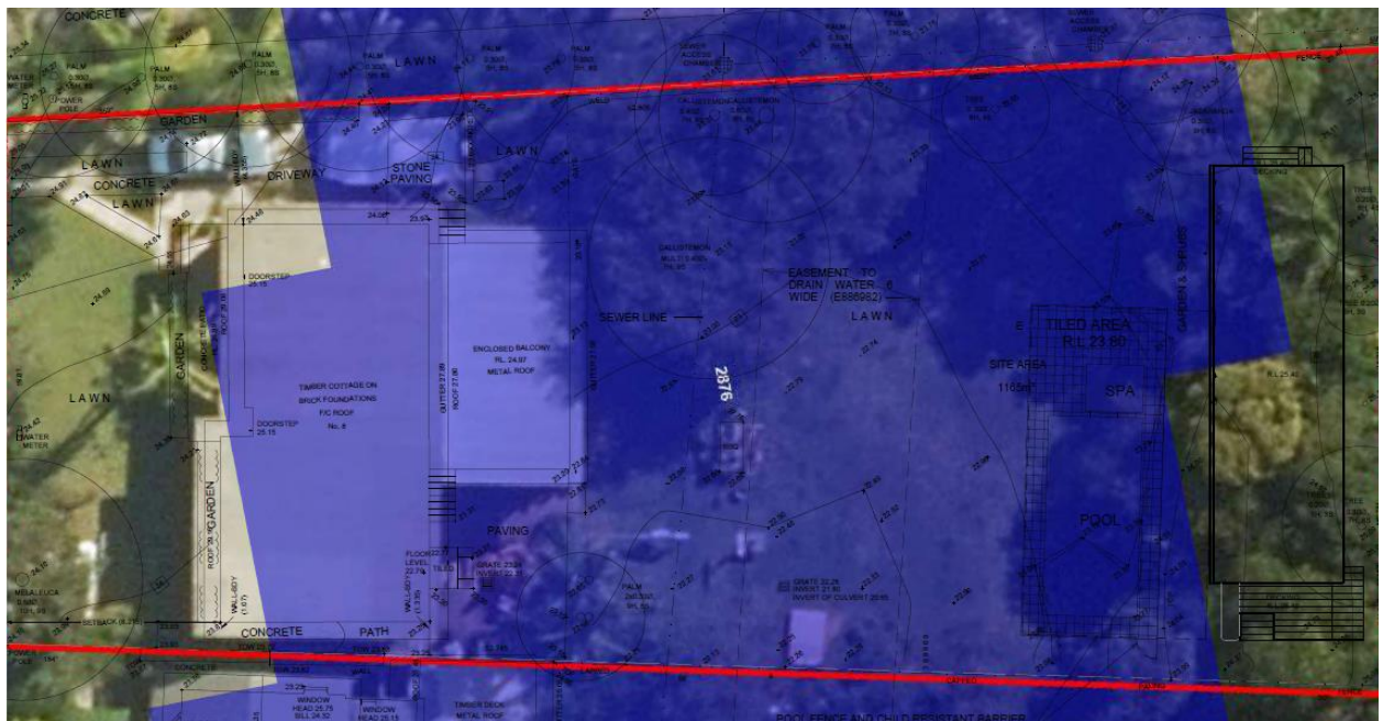
Figure 5: Ground floor plan overlay with PMF Flood Extent map
