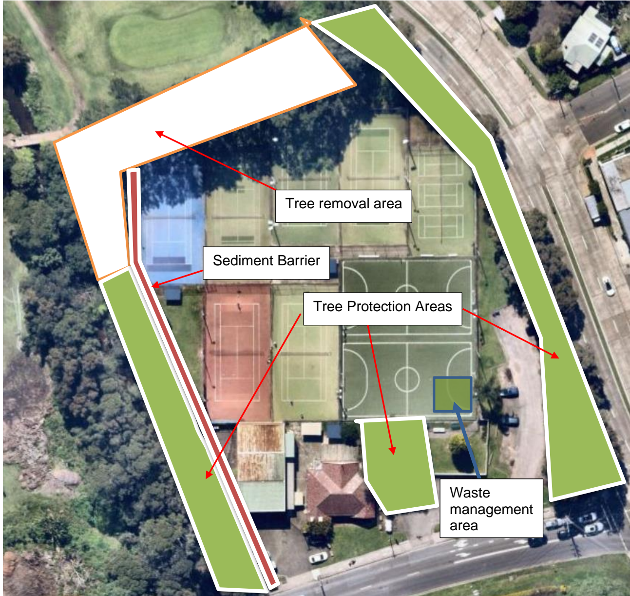
Image 9 – Tree removal and protection areas and sediment barrier positioning & waste management area.
