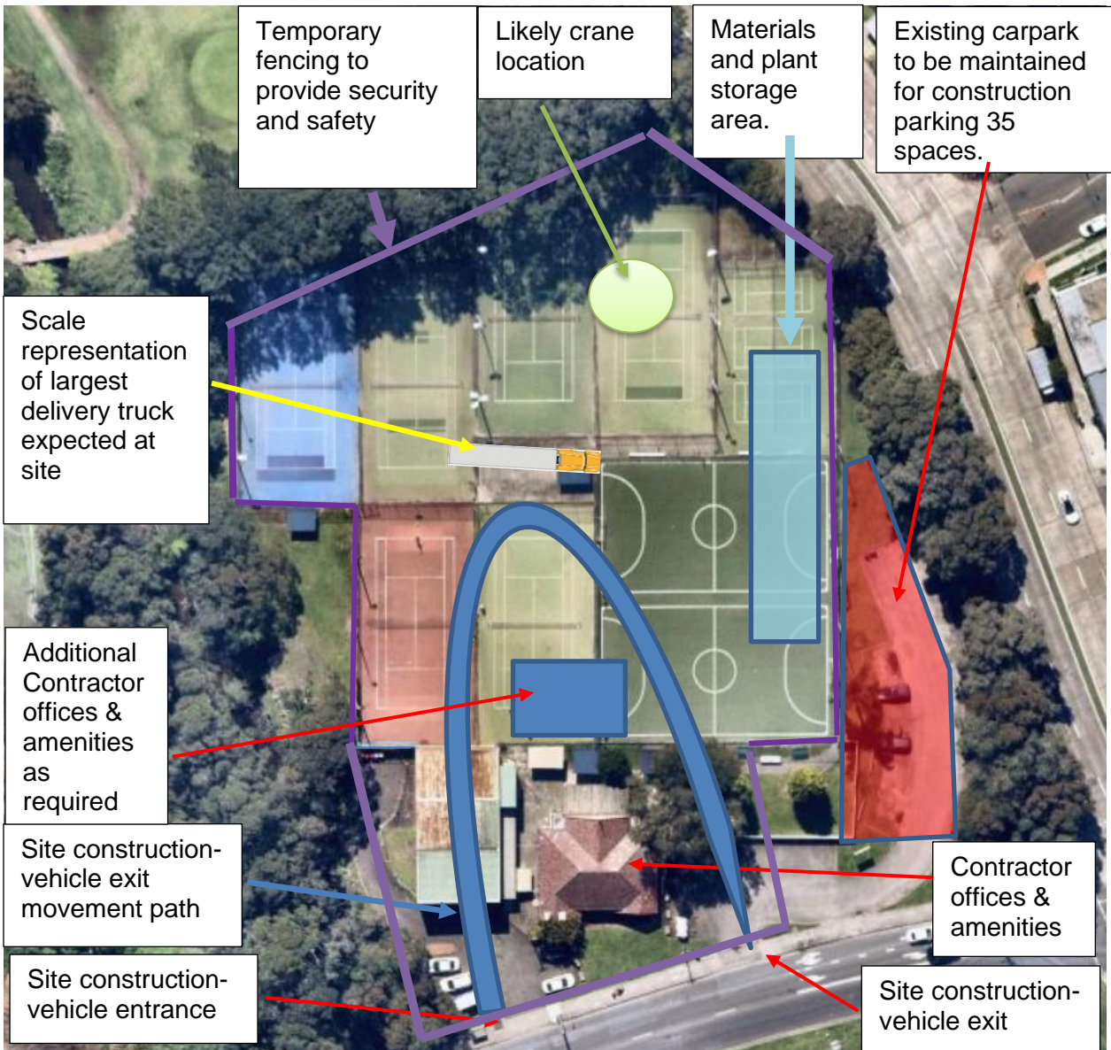
Image 6 – Security, access, crane location, and storage
