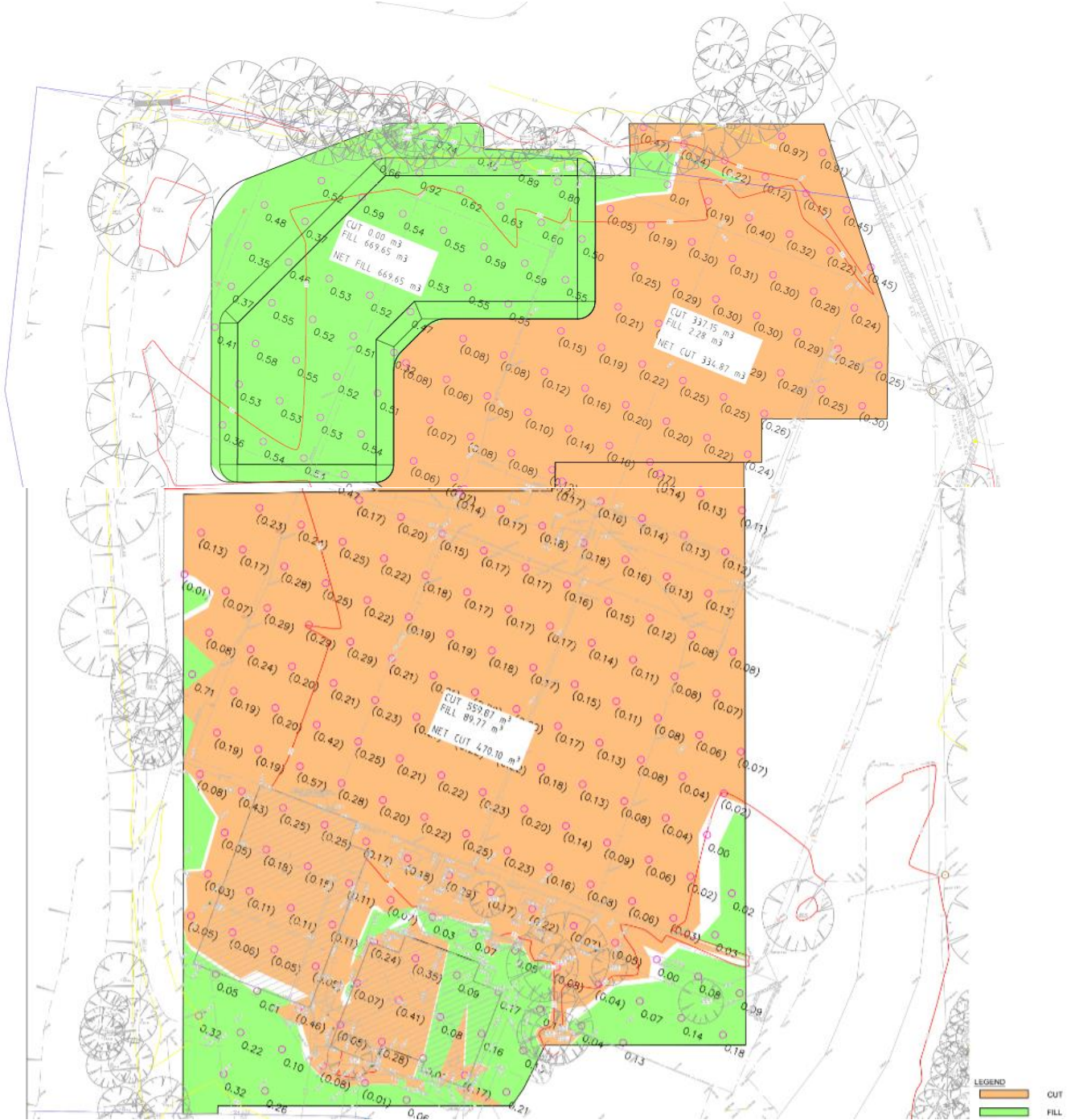
Image 10 – Excavation & Fill Plan.
