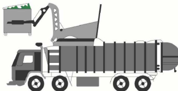
Front-lift-loading waste collection vehicle
