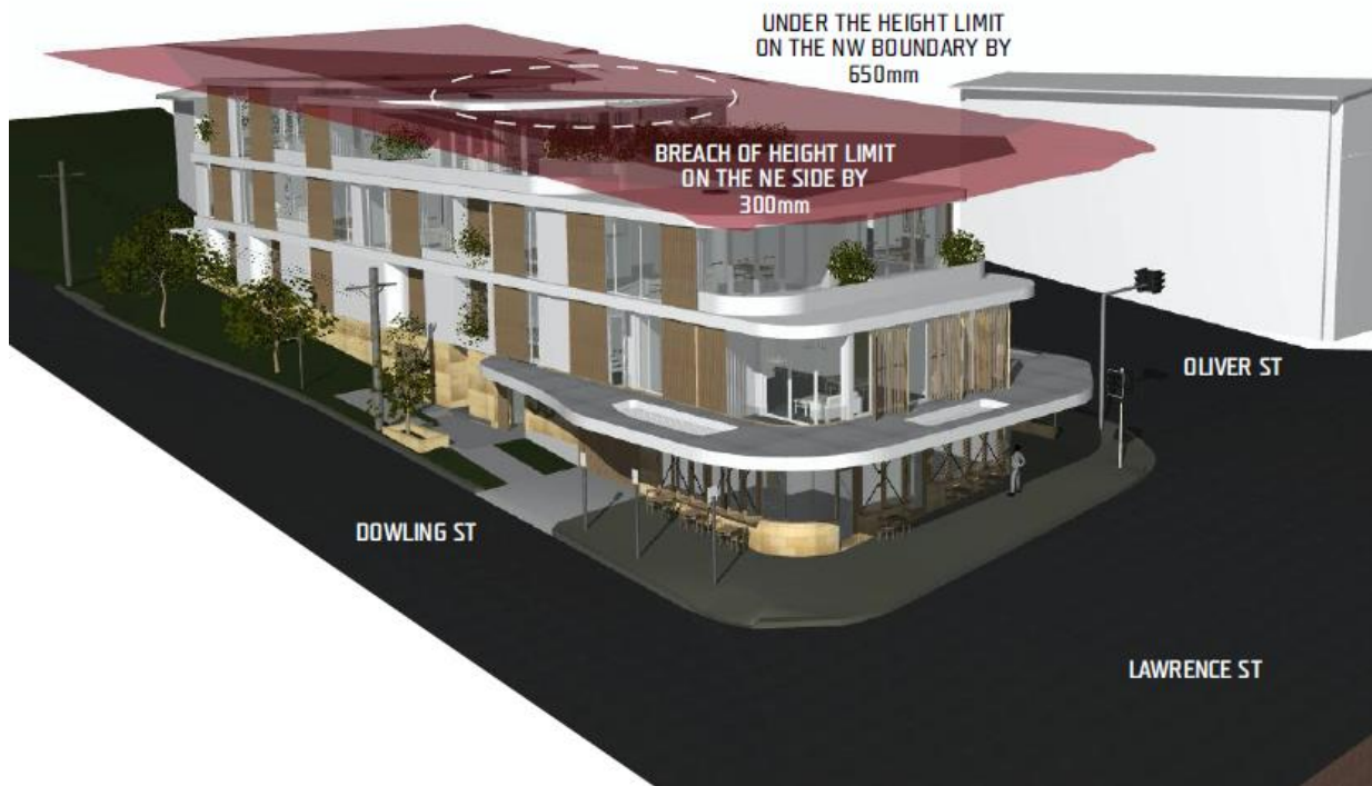
Figure 12: Plan extract showing extent of 11 metre building height breach in the north eastern corner of the roof form
