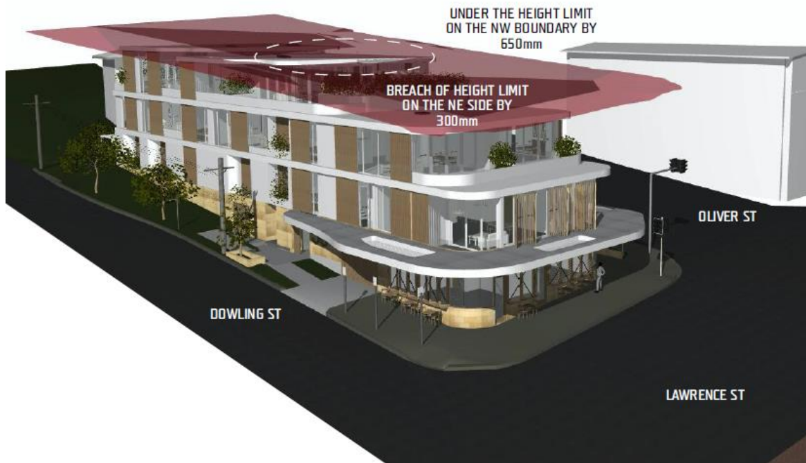
Figure 1: Plan extract showing extent of 11 metre building height breach in the north eastern corner of the roof form
