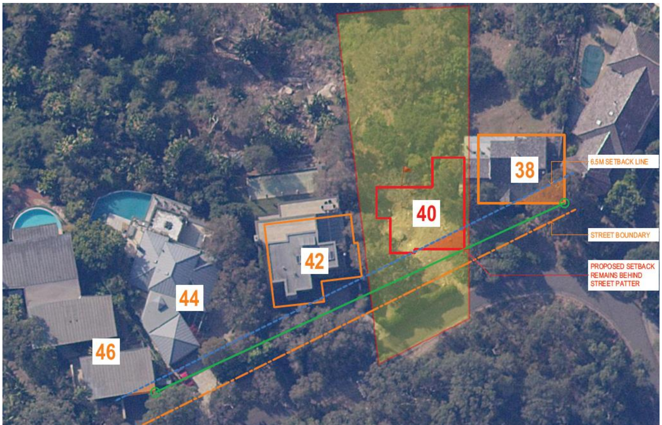
Above; Site Plan Diagram demonstrating the relationship between the proposed building envelope and the existing streetscape setback line
