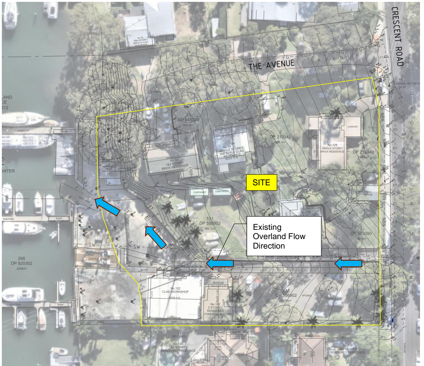
Figure 3: Existing Overland Flow Path
