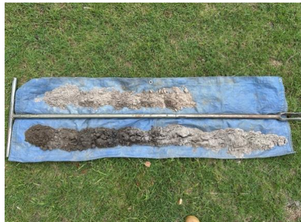
Photo 4: Subsurface soil profile seen in BH1.
