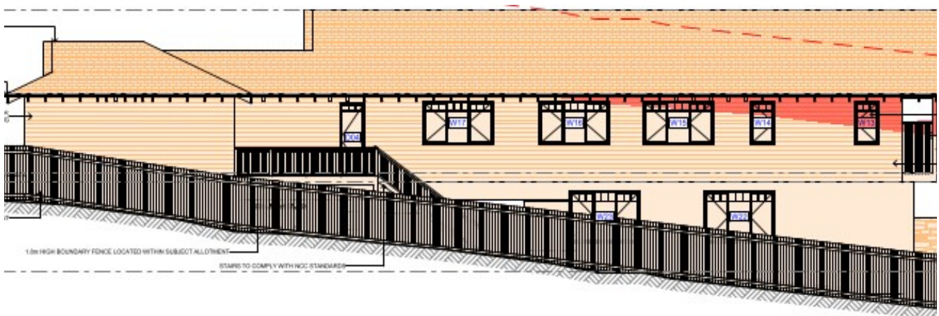
Figure 2: Extent of building envelope encroachment along the south eastern elevation shown in RED
