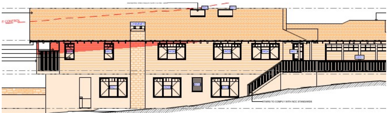
Figure 1: Extent of building envelope encroachment along the north western elevation shown in RED
