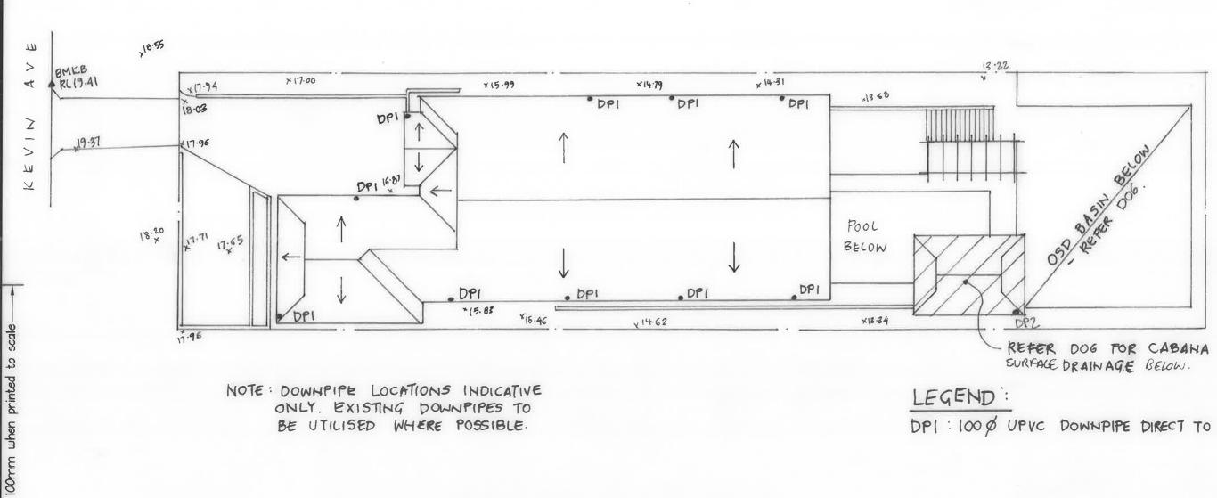
NOTE: DOWNPIPE LOCATIONS INDICATIVE ONLY. EXISTING DOWNPIPES TO BE UTILISED WHERE POSSIBLE.
