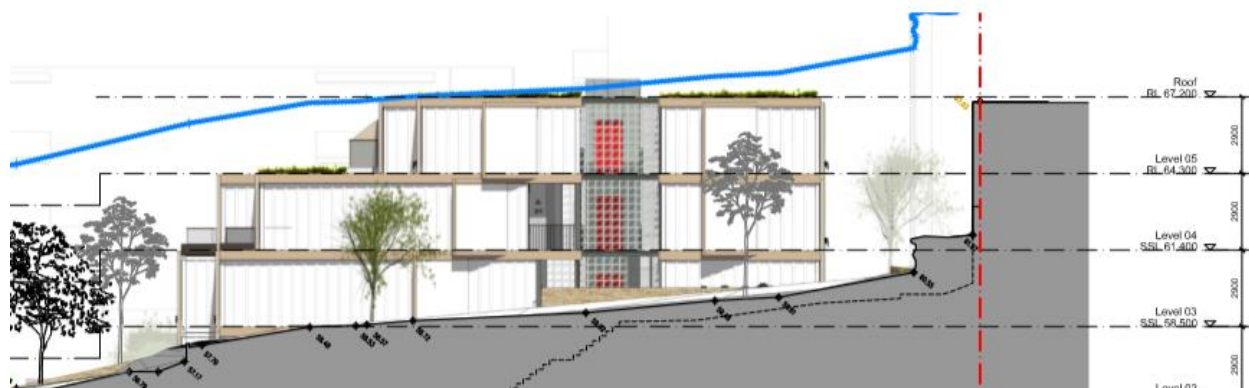
Figure 4: Extract of eastern elevation showing breach of 8.5 building height (source: Modularium Pty Ltd)
