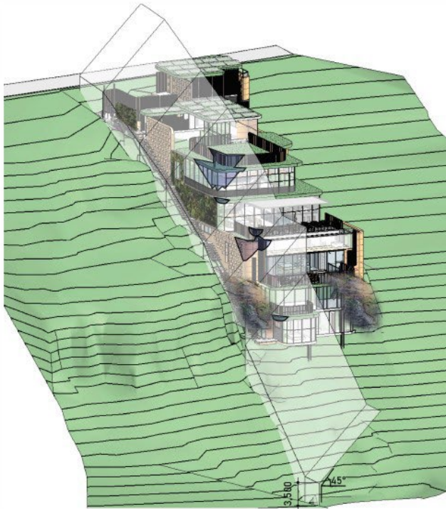
NORTHERN ENVELOPE SETBACK SHOWN AT 3.5m HEIGHT AT 45°
