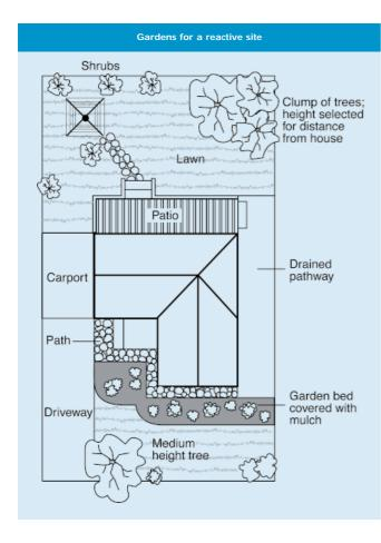
should extend outwards a minimum of 900 mm (more in highly reactive soil) and should have a minimum fall away from the building of 1:60. The finished paving should be no less than 100 mm below brick vent bases.
