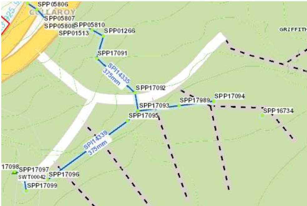
Figure 5 - DBYD existing site stormwater drainage system
