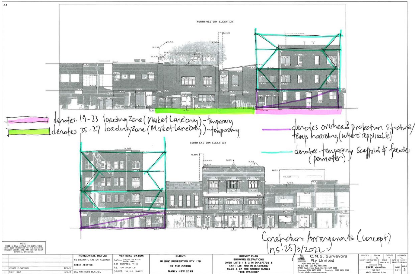
FIGURE 7 Temporary Protection arrangements
