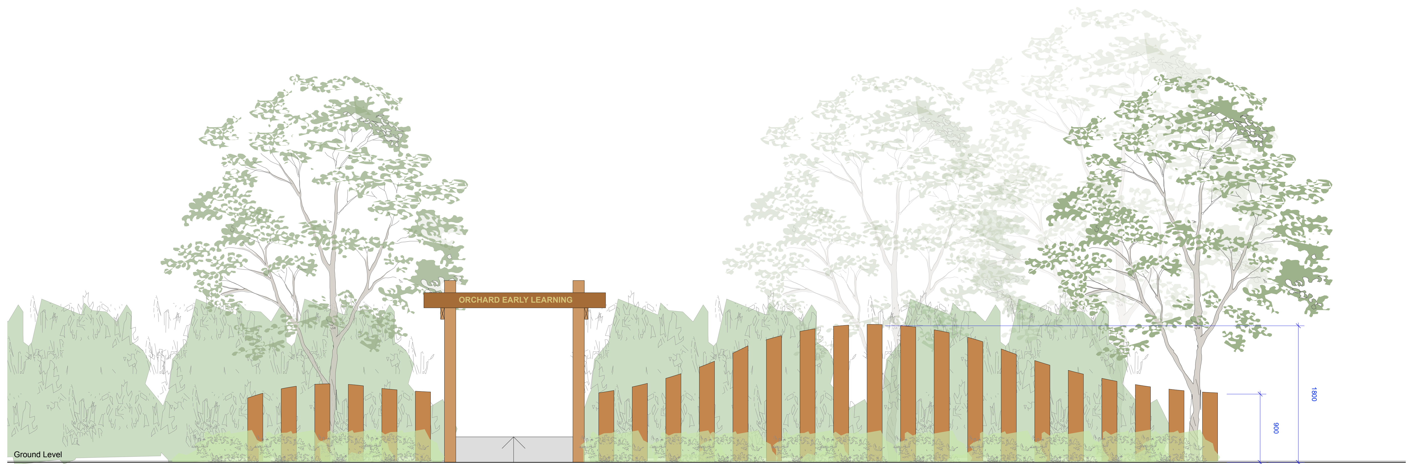
VERTICAL SLEEPER SCREEN ELEVATION 1:25
