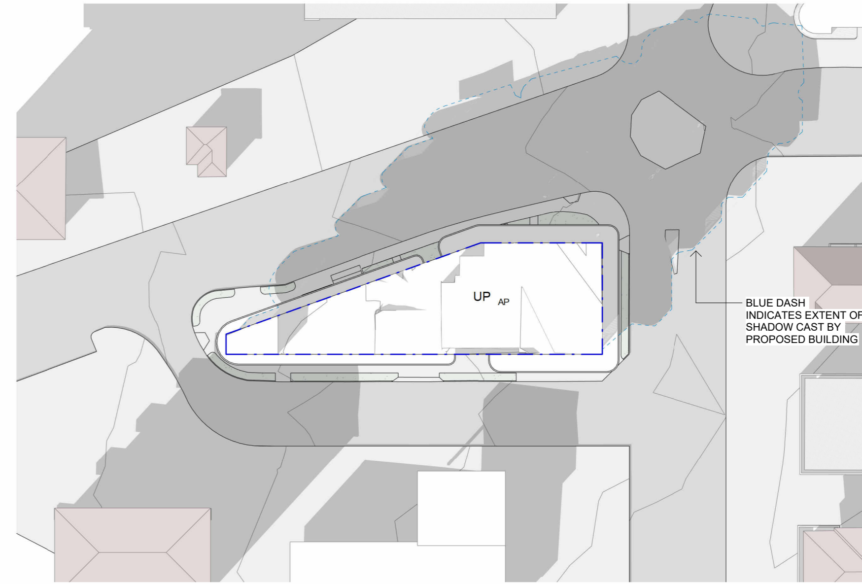
9 21 June (3pm) - Compliant Height Blanket N.T.S.
