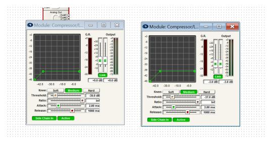
Additional controls have been installed on the powered speaker used as the main speaker system with hardware installed to remove access to additional gain controls after the limiter as shown below
