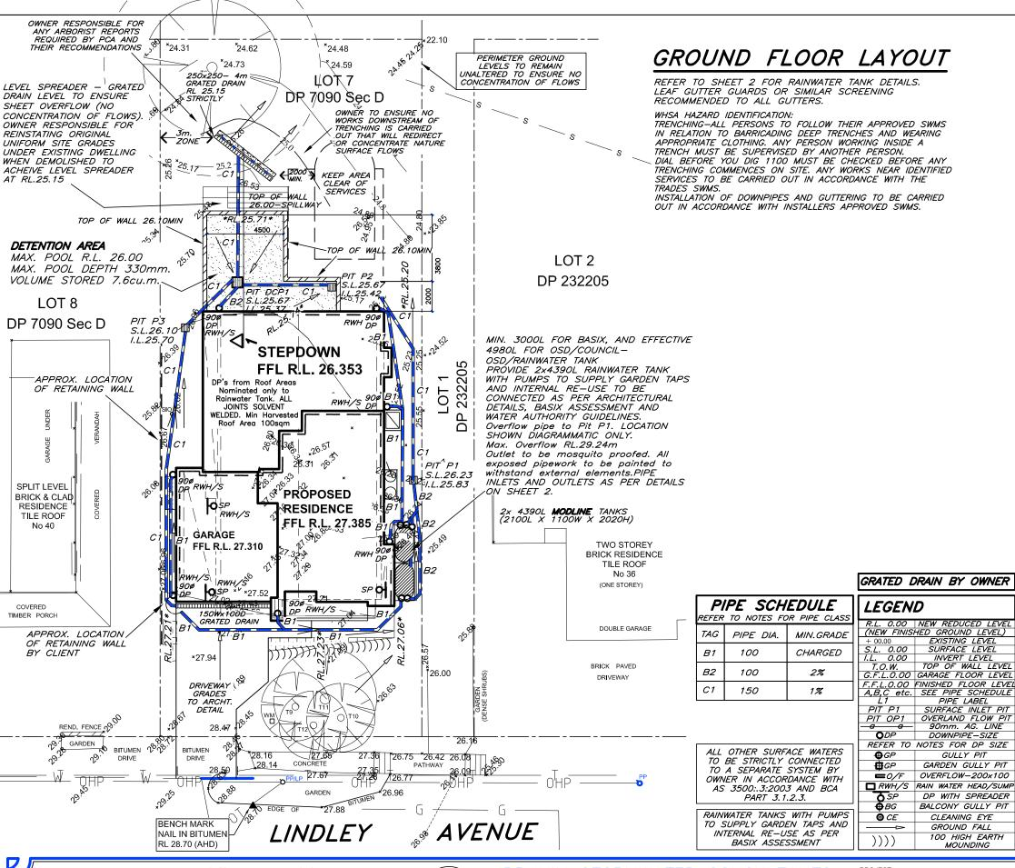
STORMWATER LAYOUT NOTES -PITS UP TO 600 DEEP TO BE 450 x 450 U.N.O., PITS UP TO 900 DEEP TO BE 600 x 600 U.N.O., PITS UP TO 1200 DEEP TO BE 900 x 600 U.N.O., PITS EXCEEDING 1200 DEEP TO BE 900 SQ. U.N.O. PITS TO BE PRECAST CONCRETE OR RENDERED BRICK WITH CONCRETE HEAVY DUTY GRATES. U.N.O. LIGHT DUTY PITS AND GRATES MAY BE USED ONLY IN LIGHT/FOOT TRAFFICABLE AREAS. U.N.O. ALL PITS TO BE BENCHED TO DISCHARGE PIPES U.N.O. GAL. STEP IRONS TO ALL PITS EXCEEDING 900 DEPTH.
