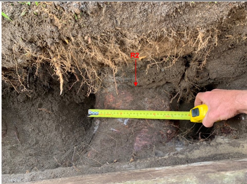
Image 6: Looking South within trench 1, showing a close up of root 2 (290mm diameter).
