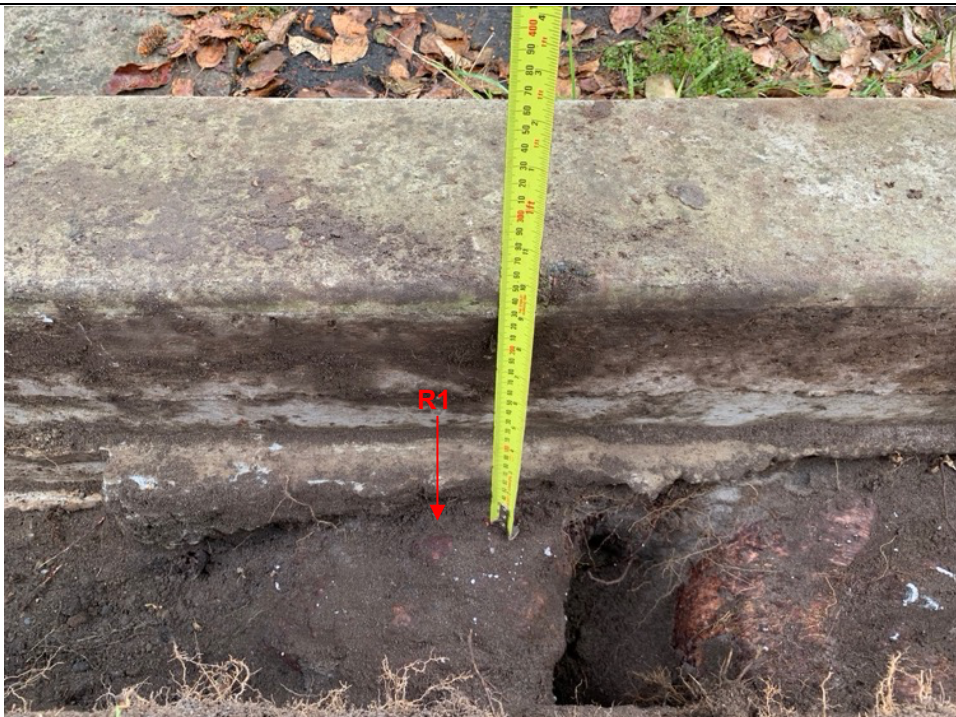
Image 10: Looking North within trench 1, showing the depth of root 1 (240mm below existing grade).
