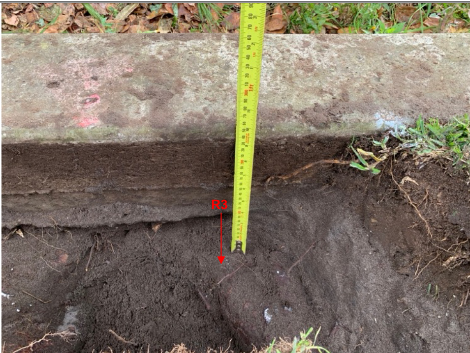
Image 12: Looking North within trench 1, showing the depth of root 3 (260mm below existing grade).
