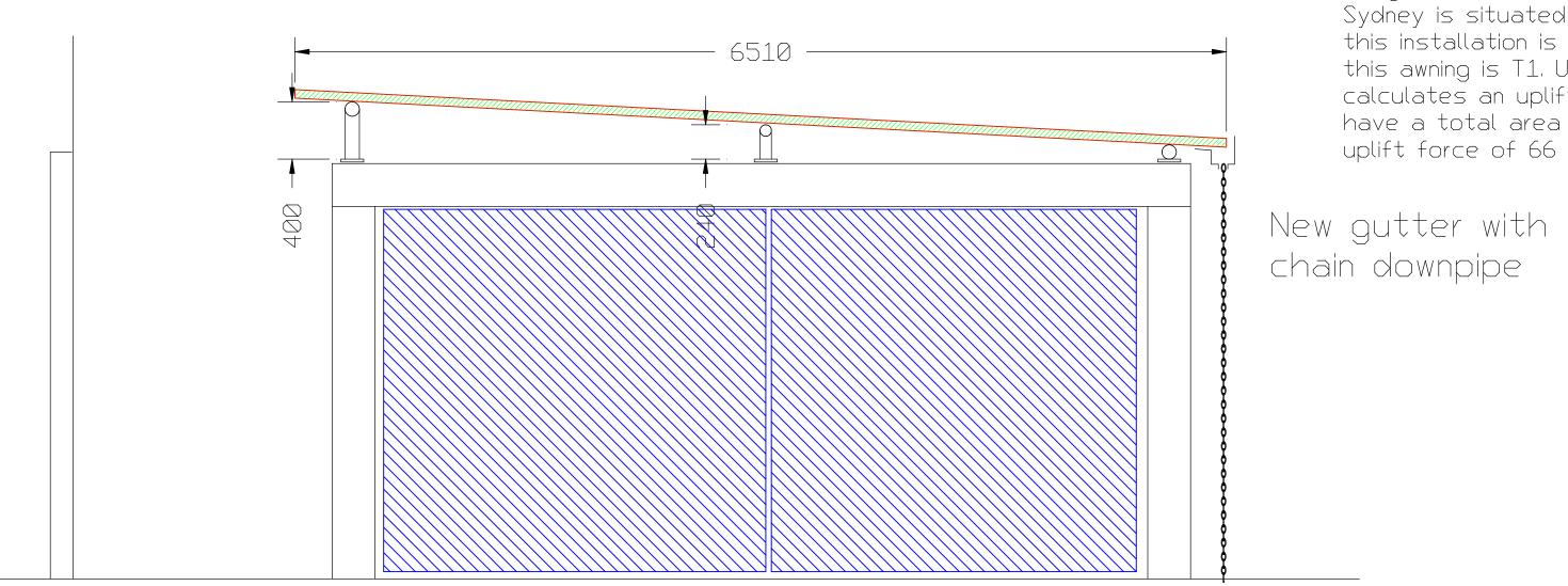
The wind loading for using Australian Stan Sydney is situated in this installation is T( this awning is T1. Usir calculates an uplift have a total area ouplift force of 66 KN
