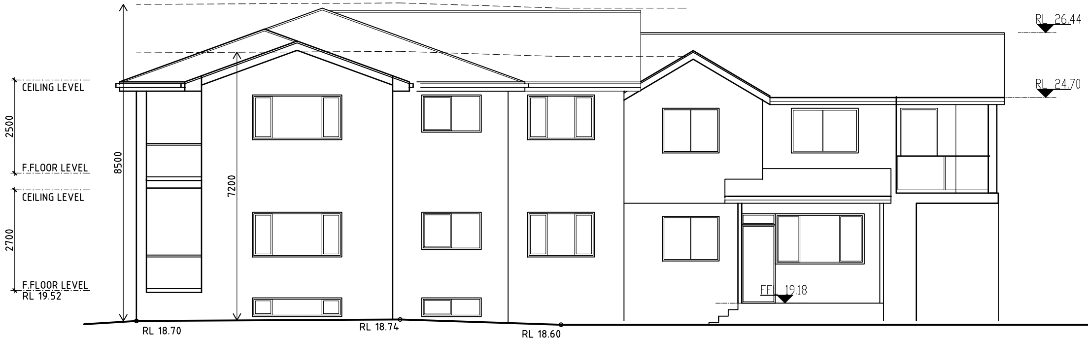
EAST ELEVATION SCALE 1:100
