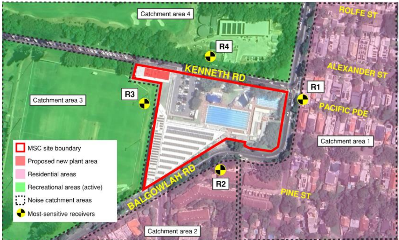
Figure 5 Most-affected noise sensitive receivers, in the context of the site and surrounding areas
