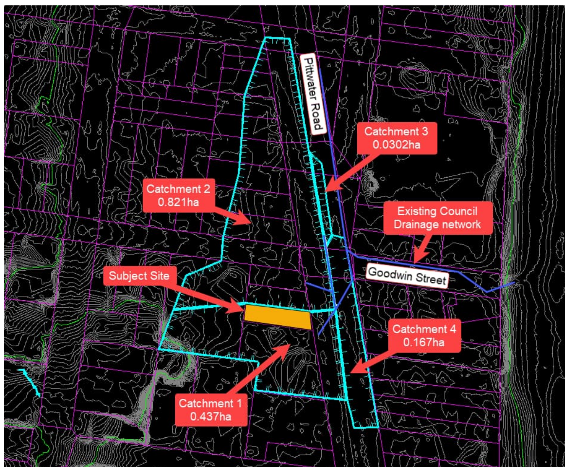
Figure 3 – Existing Catchment break-up
