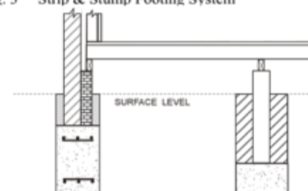
Fig. 3 Strip & Stump Footing System
