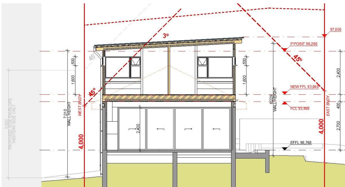
Image 3: Cross Section S2: Encroachment to Western Side Boundary Envelope
