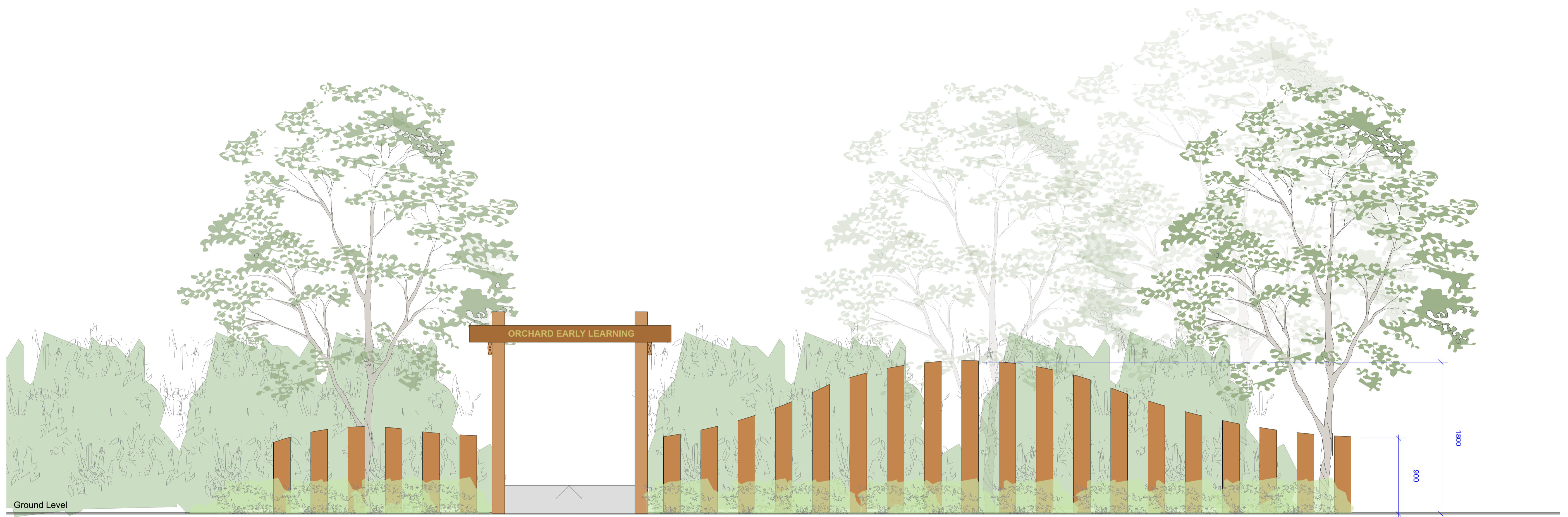
VERTICAL SLEEPER SCREEN ELEVATION 1:25
