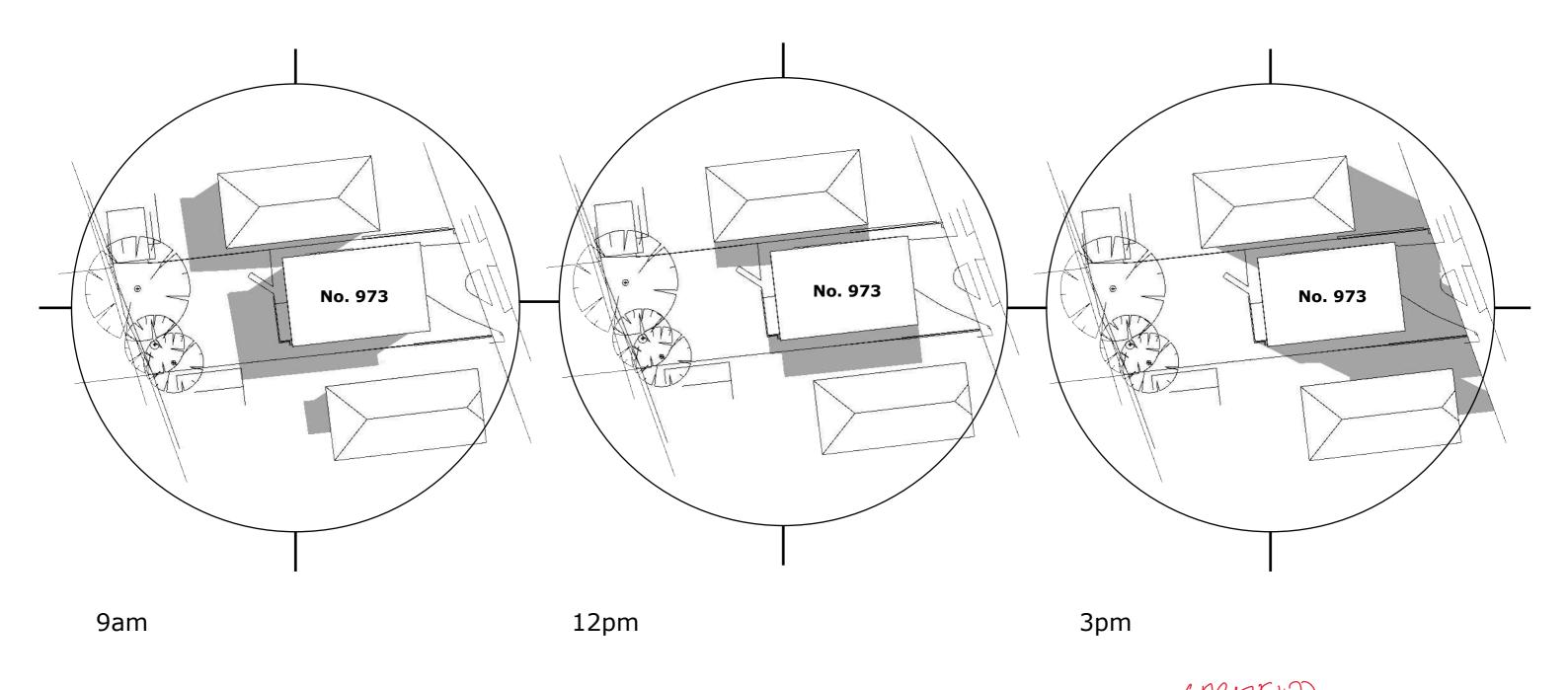
Shadow Study Diagrams - September Equinox Scale 1:500 @ A3
