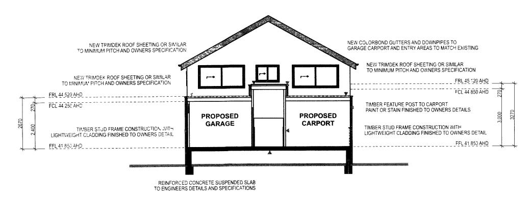
REINFORCED CONCRETE BLOCK WALL OR CONCRETE DROP BEAMS ON REINFORCED CONCRETE FOOTINGS TO ENGINEERS DETAILS AND SPECIFICATIONS
