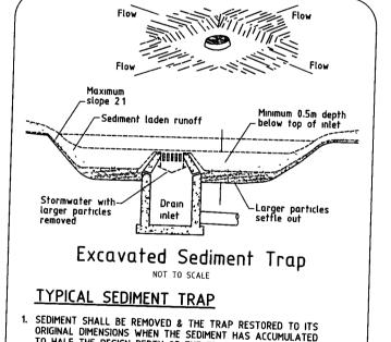
SEDIMENT SHALL BE REMOVED & THE TRAP RESTORED TO ITS ORIGINAL DIMENSIONS WHEN THE SEDIMENT HAS ACCUMULATED TO HALF THE DESIGN DEPTH OF THE TRAP. REMOVED SEDIMENT SHALL BE DEPOSITED IN A SUITABLE AREA & IN SUCH A MANNER THAT IT WILL NOT ERODE.
