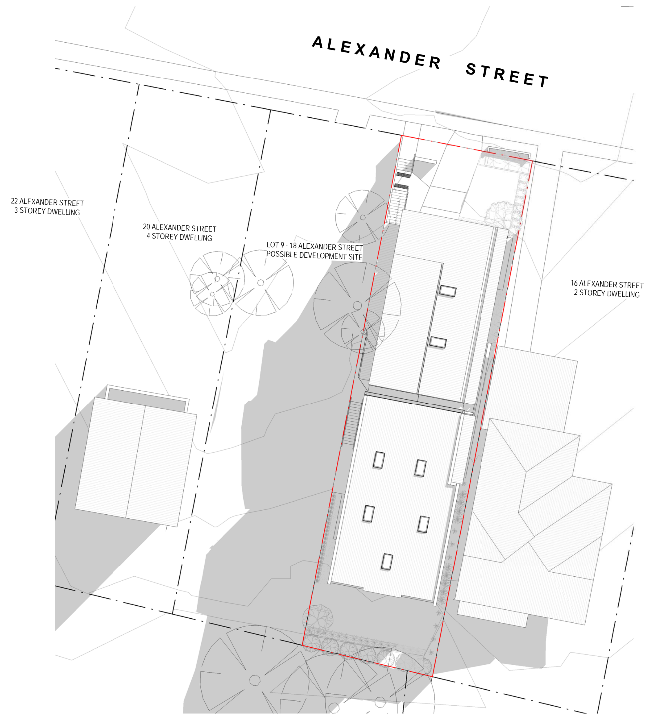
2 PROPOSED SHADOW DIAGRAM - 9AM JUNE 21ST DA500/ 1:200 @ A1
