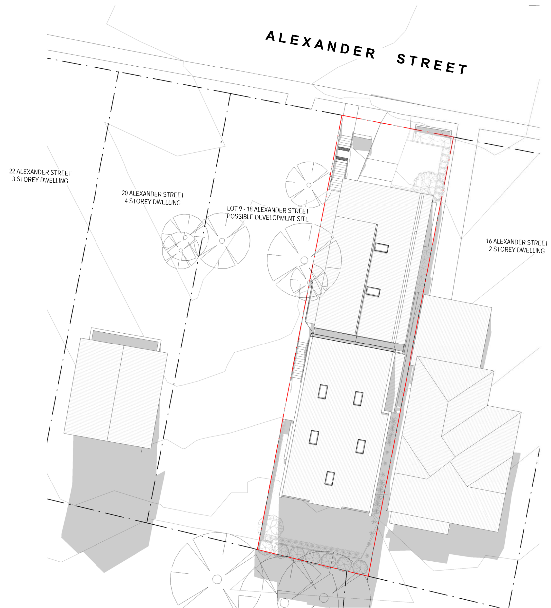
2 PROPOSED SHADOW DIAGRAM - 12PM JUNE 21ST DA502/ 1:200 @ A1
