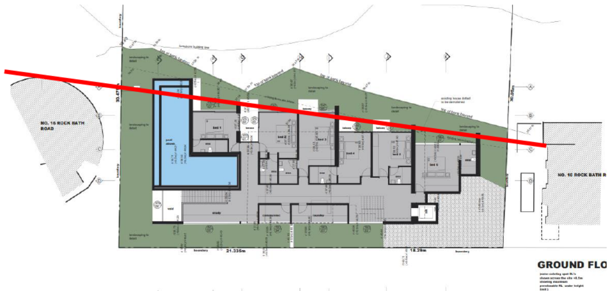
Figure 2 – Ground Floor plan with red line showing required façade alignment to maintain a view sharing outcome.
