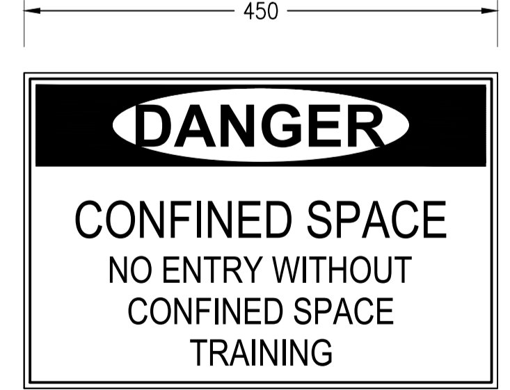
CONFINED SPACE SIGN DETAIL SCALE 1:20
