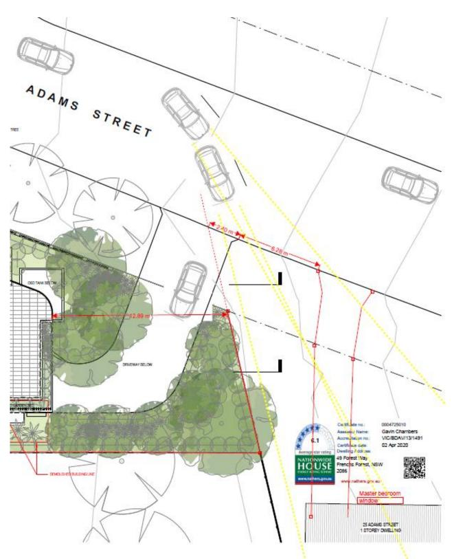
Extract from Ground Floor Plan amended and scaled in Bluebeam. Our driveway superimposed in red onto plan (not shown in submitted drawings). Vehicles turning into driveway from west will direct headlights through master bedroom and living room windows. Driveway extends 2.4m past our shared boundary position, driveway only 6m from our driveway.
