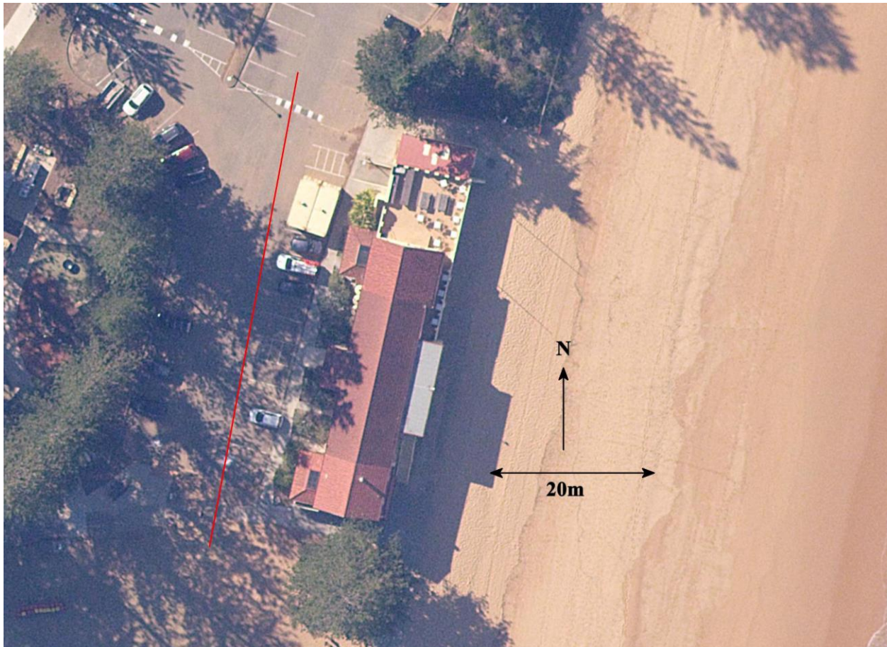
Figure 16: Position of coastal erosion acceptable risk line for immediate planning period at Newport SLSC
