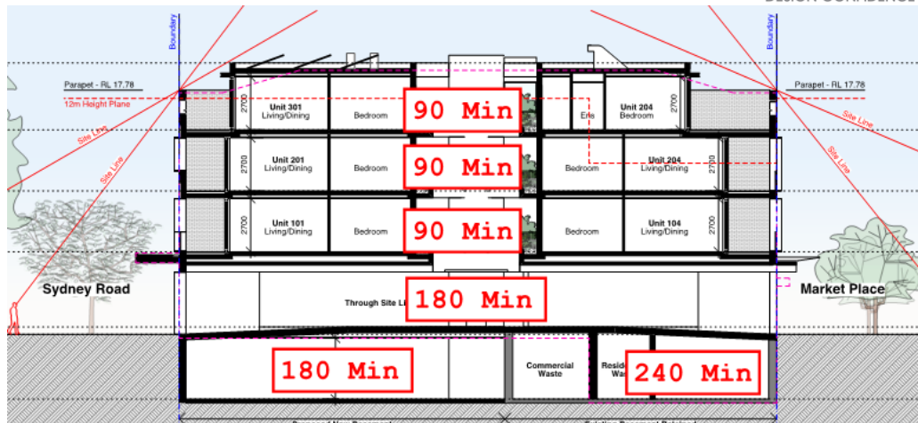
Figure C2.9 – Separation of class 2, 6 and 7b between storeys
