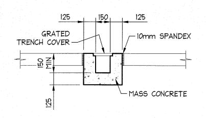
OR PRECAST GRATED DRAIN ALTERNATE POLYPROPYLENE DRAIN BY MANUFACTURER
