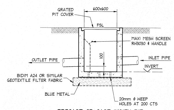
PRECAST OR CAST INSITU PIT REFER STORMWATER NOTES ALTERNATE POLYPROPYLENE PIT BY MANUFACTURER
