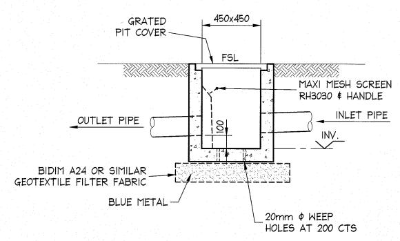
PRECAST OR CAST INSITU PIT REFER STORMWATER NOTES ALTERNATE POLYPROPYLENE PIT BY MANUFACTURER
