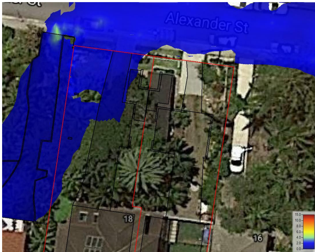
Figure 9 Flood Velocity for Existing Condition in 1% AEP Storm
