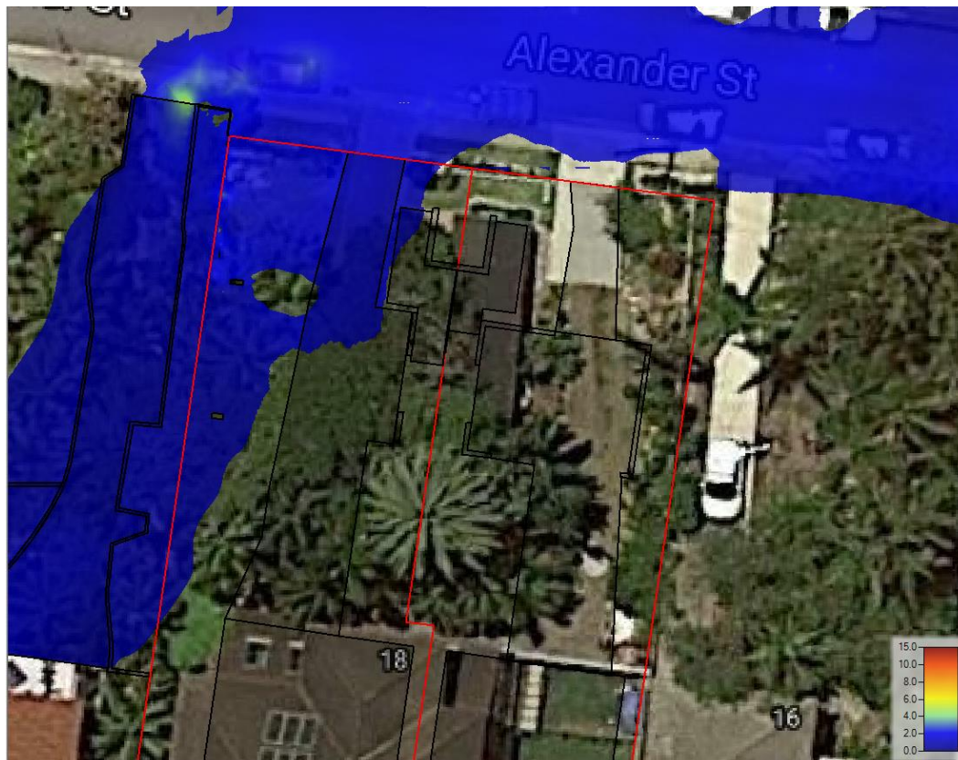
Figure 12 Flood Velocity for Developed Condition in 1% AEP Storm
