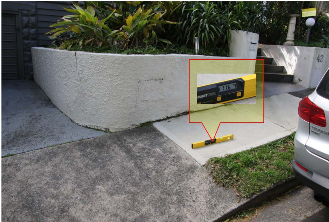
Photo 2.1: Gradient of the footpath adjacent to the existing footpath (Photo: traffic Engineering Centre Pty Ltd)
