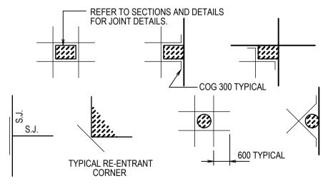
SLAB ON GROUND - ALL TRIMMERS TO BE 2N12 TOP U.N.O. SUSPENDED SLAB - ALL TRIMMERS TO BE 3N16 T&B U.N.O. TYPICAL TRIMMER DETAILS AT ALL COLUMNS, WALLS, PITS, FLOOR WASTES, ETC THAT CAUSE A PENETRATION THROUGH THE SLAB.
