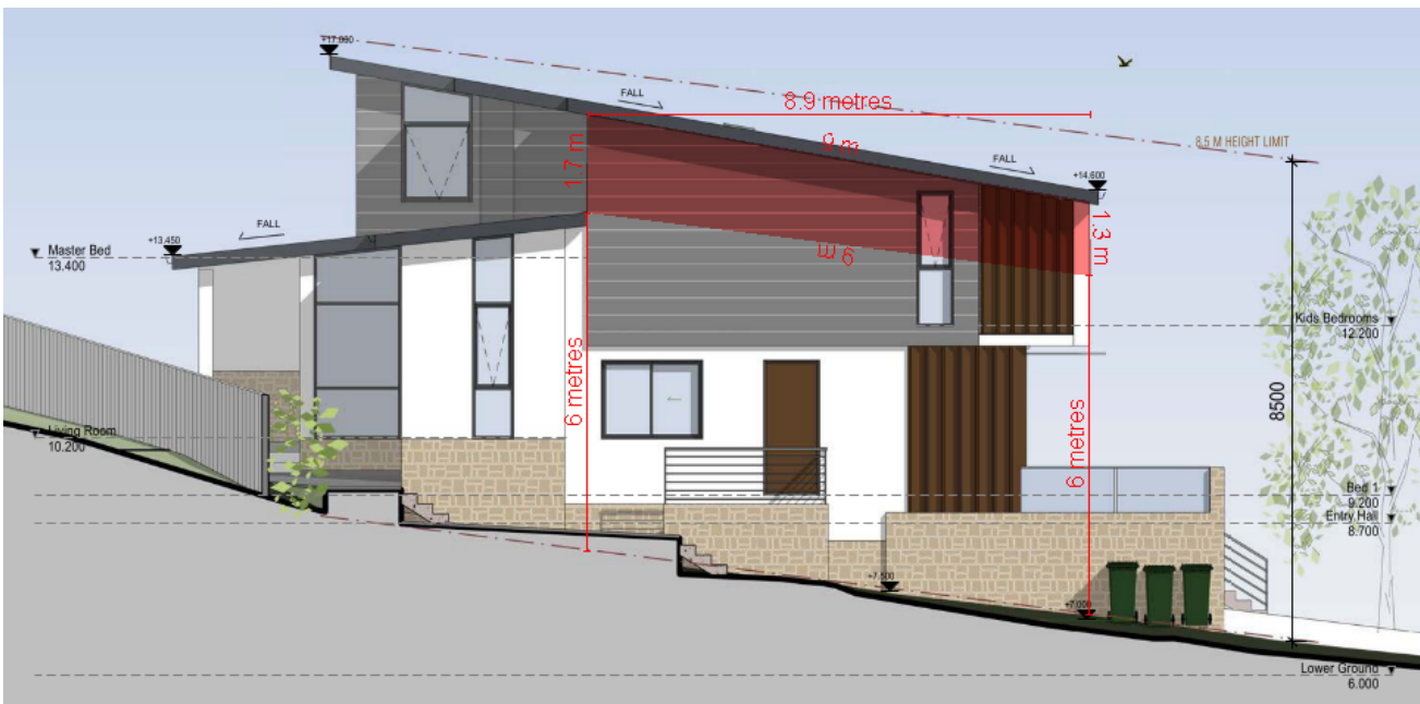
Figure 2 - Extract from West Elevation with envelope breach in red.
