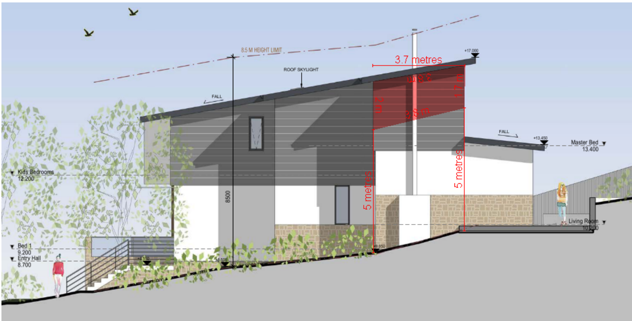
Figure 3 - Extract from East Elevation with envelope breach in red.
